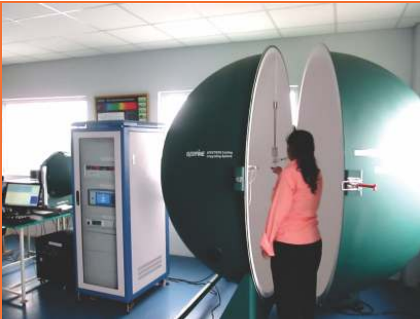
Integrating Sphere and Photometric Testing Laboratory
